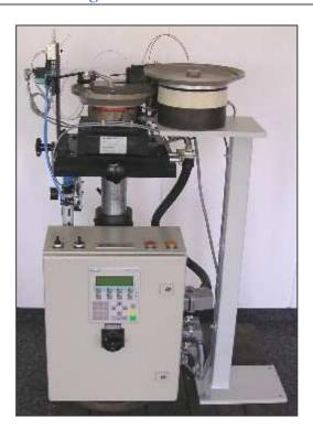
The WF82 filament feeder has for many years been a well appreciated equipment to feed filaments.
