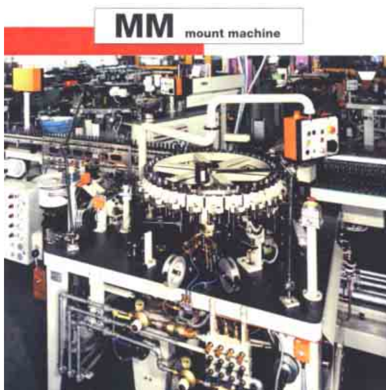
mounting the filament on pinched stems
