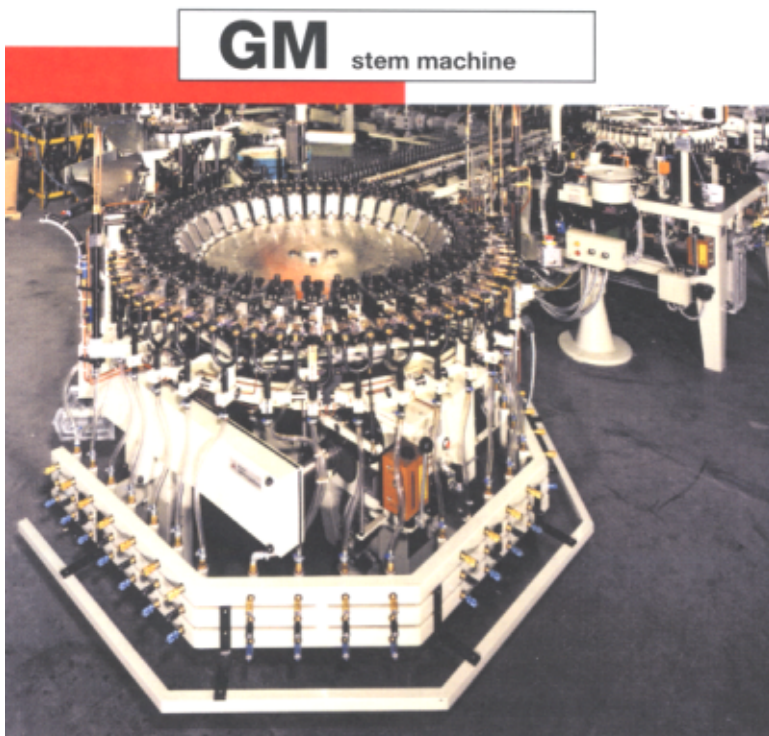
producing the pinched stems
