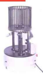
This machine is used for cutting yods and exhaust tubes for the production of incandescent lamps. Its design is simple and its production rate high.
