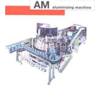
The aluminizing machine has been designed for the internal coating of bulbs for reflector lamps, crown mirrored lamps and PAR reflector lamps by evaporation of an aluminum wire.
