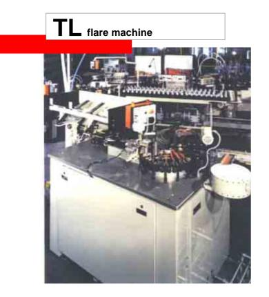
The TL machine is used for the production of flares for the manufacture of incandescent lamps. The machine consists of two parts, an automatic tube loading and cutting system and a horizontal flaring turret.
